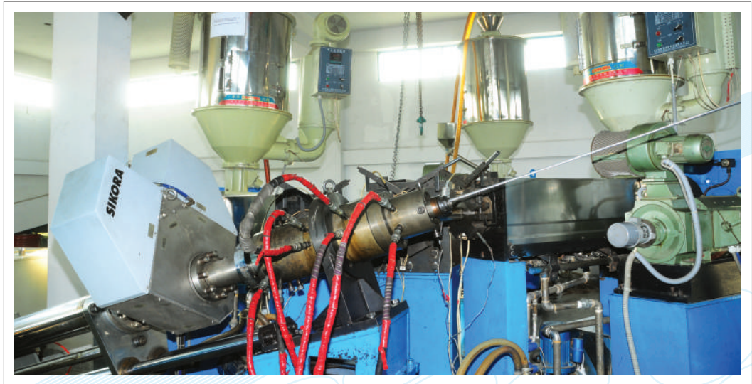
View of Triple Extrusion Line with SIKORA of Germany
